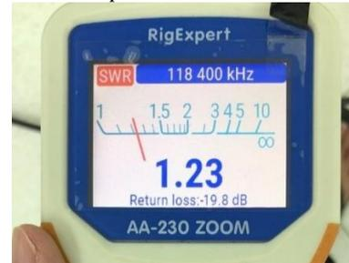
Gambar 11. VSWR Antena *Yagi*
