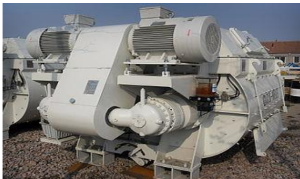
Twin shaft concrete mixer for concrete plant
