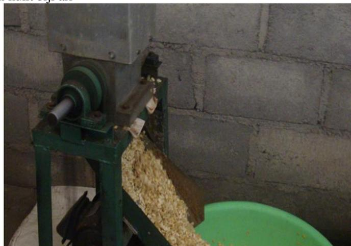
Gambar 4 Proses Pengupasan Kulit Biji Ari
