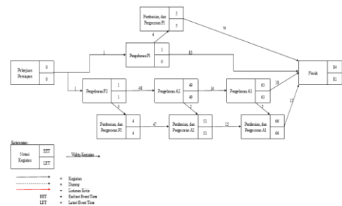
Gambar 4.6 Diagram Network Planning Pekerjaan Bore Pile Alternatif 1
