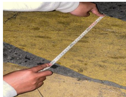
Gambar 4.2. Pengukuran Marka Yellow Box Junction
