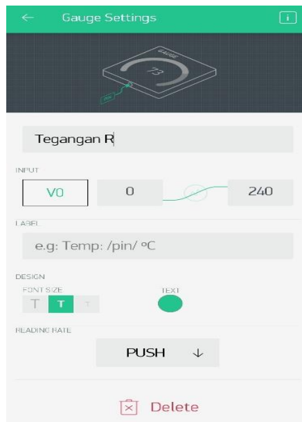
Gambar 3.7. variable system blynk fasa R
