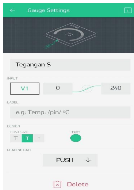
Gambar 3.8. variable system blynk fasa S
